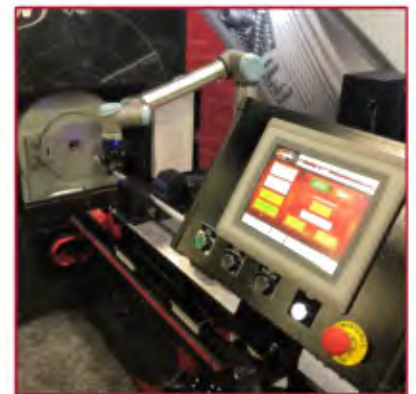
Example of a FENN Turn-Key Automated Swaging Solution: FENN Swager, Sound Enclosure, Feeding System, & Integrated Automation.
