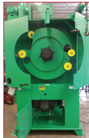
Dead Block Rebuild After
